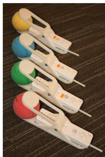
Figure 7 Four 3D printed Pipet add-ons with Nintendo WiiMotes
