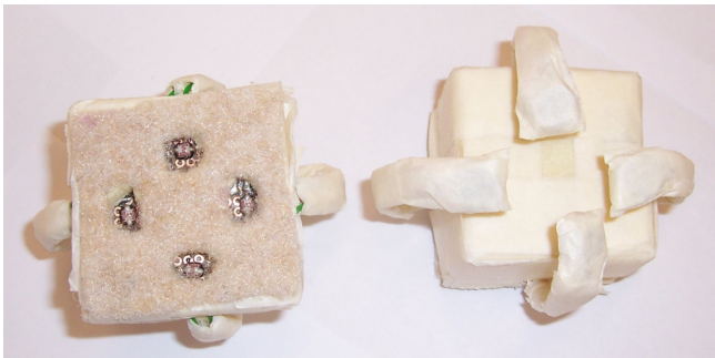
Figure 4. The fifth prototype's bottom (left) and top (right). During a game the player covers the top with his hand.
