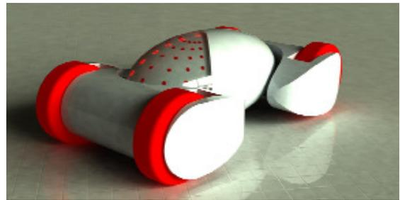
**Figure 3.** The design of the battle-tank: with LEDs providing feedback about the aiming direction.
