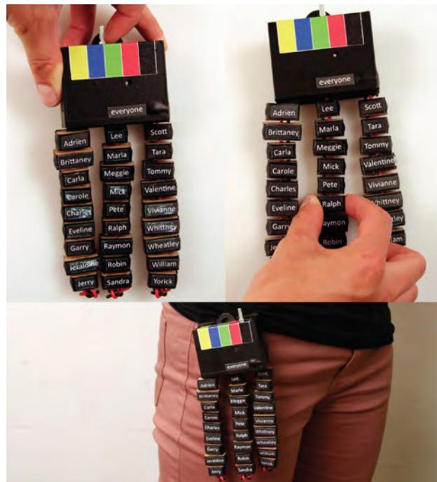
**Figure 2.** FireFlies Teacher-Tool: selecting a colour (top left), selecting a child's name (top right) and clipped to the user's clothes (bottom)
